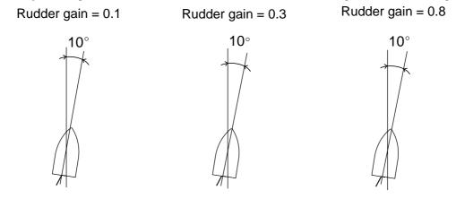
Rudder angle =  $10^{\circ} x \ 0.1=1^{\circ}$  Rudder angle =  $10^{\circ} x \ 0.3=3^{\circ}$  Rudder angle =  $10^{\circ} x \ 0.8=8^{\circ}$ Rudder angle and rudder gain setting
